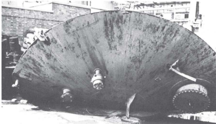
FIGURE 5-10 When an explosion occurred in a tank, the roof landed on an area just big enough to contain it.
