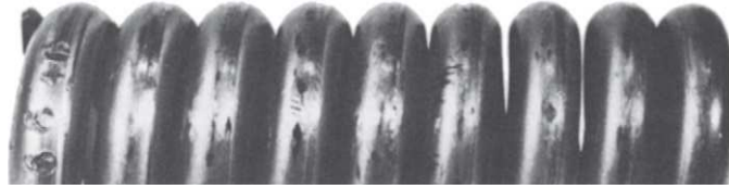
FIGURE 10-9 Example of too many coils.
