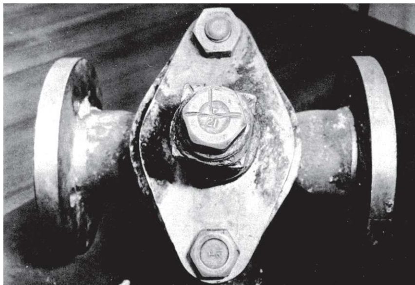
FIGURE 25-3 The central bolt was marked to show the position of the cock. When two washers were inserted under the bolt, it could not be screwed down as far as before and the marks no longer corresponded with the position of the cock.
