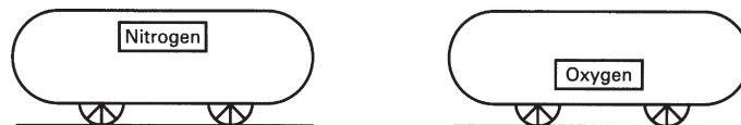
FIGURE 4-2 Arrangement of labels on tank cars. The Nitrogen label folds down to read Oxygen.
