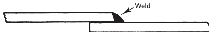
FIGURE 5-11 An old method of tank construction allows liquid to enter the gap between the plates.
