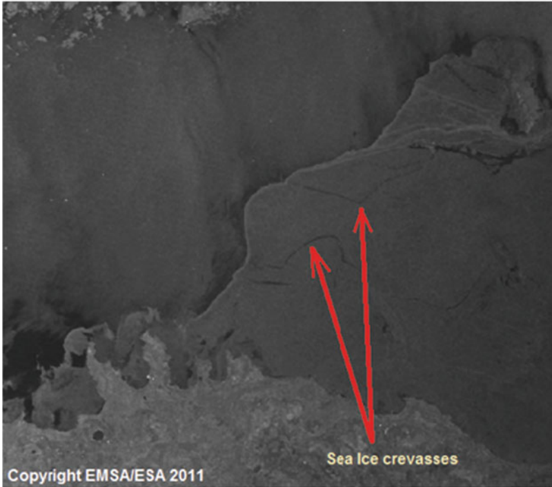
Fig. 6 Envisat ASAR image on 20/04/2011 at 08:56 UTC over the Gulf of Finland. In this case the dark patches pointed by the arrows are a low backscatter area inside a block of sea ice. It is important to locate the sea ice areas to avoid misclassification. The boundary between the sea ice and the open sea offers a bright feature that turns into dark in the open water
