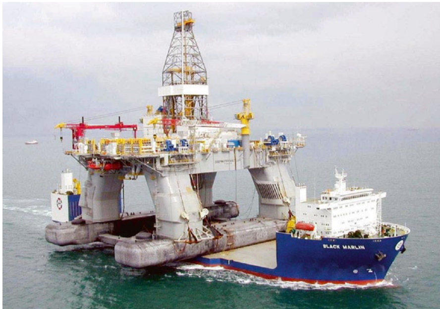
Fig. B.3 The Deepwater Horizon was a semi-submersible drilling rig capable of operating in harsh environments and water depths up to 8,000 feet (upgradeable to 10,000 feet) using 18-3/4 inch, 15,000 psi blowout preventer (BOP) and 21 inch, OD marine riser. The rig could drill to the maximum water depth of 30,000 feet/9,144 meters. It displaced 8,000 metric tonnes of water and was 396 feet/121 meters long, 256 feet/78 meters wide, and 136 feet/41 meters deep. (Source: Transocean, http://www.nytimes.com/2010/12/26/us/26spill.html )
