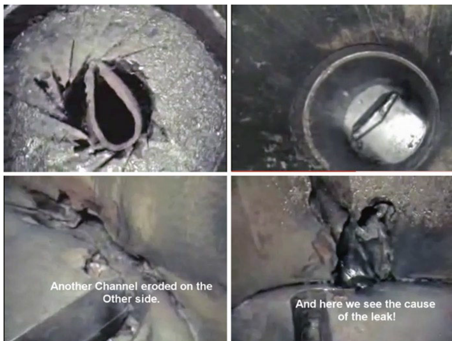
Fig. 7.6 Four frames from a video of an inspection of the Macondo well Blowout Preventer lifted up by the Helix Q4000 vessel on November 6, 2010. From the upper-left, clockwise, the fiber-optics video camera shows (1) the closed annular preventer with a drill pipe crimped in, (2) the almost-closed and eroded blind shear ram below, (3) erosion channels on one side of the ram, and (4) on the other side of it. Reservoir oil and gas flowed through a narrow slit in the ram and etched the hard steel shears. The video was leaked to YouTube, www.youtube.com/watch?v=UxCt3UsmJF0
