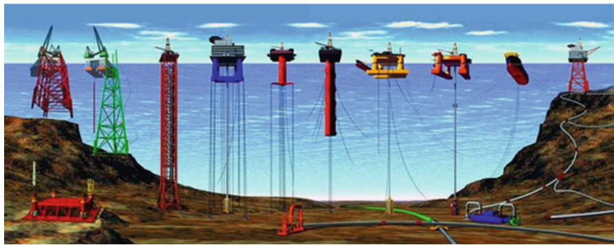
Fig. 4.3 Types of offshore oil and gas structures include (Bottom figure from left to right): Two conventional fixed platforms (deepest: Shell’s Bullwinkle in 1991 at 412 meter/1,353 feet, GOM); a compliant tower (deepest: ChevronTexaco’s Petronius in 1998 at 534 meter/1,754 feet, GOM); two vertically moored tension leg and mini-tension leg platforms (deepest: ConocoPhillips’ Magnolia in 2004, 1,425 meter/4,674 feet, GOM); a spar platform (deepest: Dominion’s Devils Tower in 2004, 1,710 meter/5,610 feet, GOM); two semi-submersibles (deepest: Shell’s Perdido in 2010, 2,438 meter/8,000 feet, GOM); a floating production, storage, and offloading facility (deepest: 2005, 1,345 meter/4,429 feet, Brazil); a sub-sea completion and tie-back to host facility (deepest: Shell’s Coulomb tie to NaKika 2004, 2,307 meter/ 7,570 feet. In 2009, the deepest reeled flowline installation at a water depth of 2,961 meter (9,713 feet) was Shell’s Perdido, GOM). Sources: Office of Ocean Exploration and Research, National Oceanic and Atmospheric Administration; Shell
