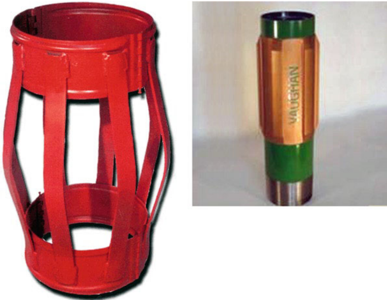
Fig. 4.7 Left: A typical casing centralizer with two collars that are screwed onto a string of casing tube. Right: A more sophisticated version of the centralizer on the left is a “centralizer sub,” that can be screwed in-between two strings of casing, thus providing greater mechanical integrity (the centralizer collars cannot slip and lock casing in the hole at some intermediate depth). The BP engineers on the Deepwater Horizon did not like centralizers like the one on the left, thought that they did not have enough of the subs on the right, and installed only six centralizer subs, as opposed to 21 or so that were needed according to Halliburton. (Sources: Bond-Coat, Inc., Midland, TX; and Casing Systems International, LLC, Scott, LA)
