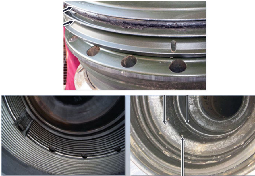
Fig. 7.5 Top: The production casing hanger seal assembly from the outside. Apparently, the Macondo well casing did not move up and then drop down, because the seal is intact, as the two arrows indicate. Also, if the reservoir fluid flowed through the annular space, it would have to exit through the small holes on the perimeter of the assembly. The four visible holes are not eroded. Bottom: An image of the inside of a new casing hanger assembly ( left ) and in the Macondo well ( right ), showing significant erosion due to flow through the production casing. The bottom arrow shows the eroded square tab on the left. The upper two arrows highlight the extent of erosion of the grooves in the hanger. (Image source: Pages 118 and 119 of the presentation based on the Deep Water – The Gulf Oil Disaster and the Future of Offshore Drilling , Report to the President, National Commission on the BP Deepwater Horizon Oil Spill and Offshore Drilling)
