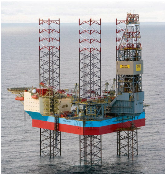
Fig. B.2 Mærsk Inspirer, one of two identical rigs sharing the title of being the world's largest and most advanced harsh environment jack-up rigs. (Source: www.maersk-drilling.com )
