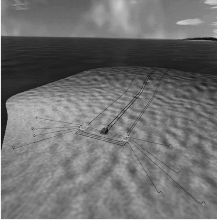
Fig. B.9 A sea-to-shore production system does not need a fixed platform. (Source: NOAA, the photo is courtesy of Mystic Aquarium/IFE)
