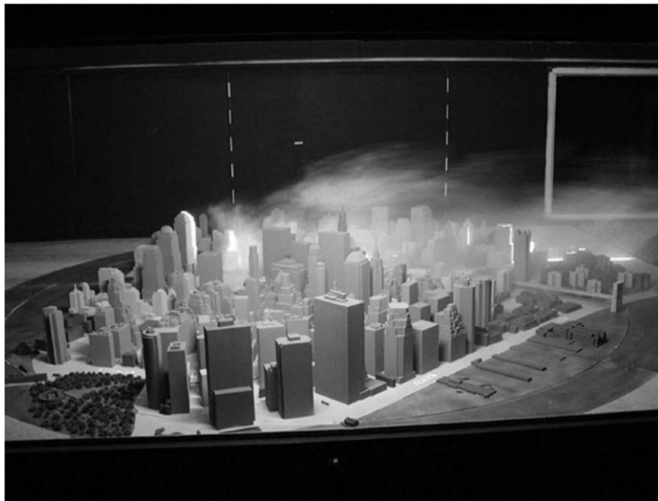
FIGURE 4.2 Example of a simulated plume of neutrally buoyant smoke released from the World Trade Center; using a physical wind-tunnel model, flow from left to right is displayed; natural light is illuminating the smoke and a vertical laser sheet is additionally illuminating the plume near the centerline of source. Vertical laser sheet is additionally illuminating the plume near the centerline of source. Photo used with permission from: U.S. Environmental Protection Agency. Perry S, Heath D. Fluid modeling facility. North Carolina: Research Triangle Park; 2006.
