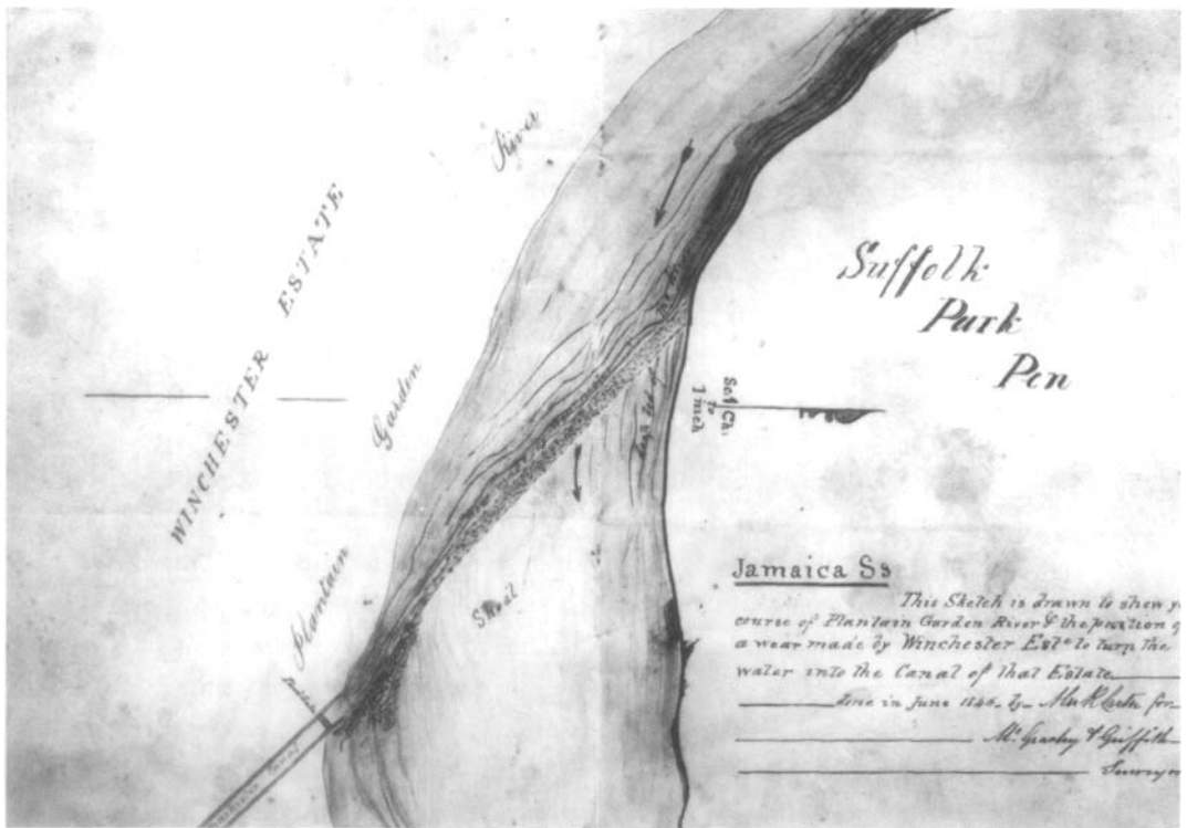
Figure 7.10 "A Sketch drawn to show the course of the Plantain Garden River and the position of a weir made by Winchester Estate to turn the water into the canal of that Estate, done in June 1846 by Alexander R. Carter for McGeachy and Griffiths, surveyors". National Library of Jamaica, Plans, St Thomas 3A.
