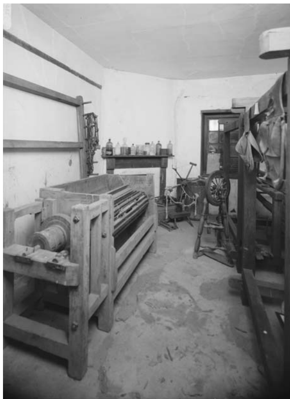
Interior of weaving house, ca. 1821, showing remains of a cotton gin. The gin is thought to have been made locally in the 19th century by William Ellison, a free black carpenter and entrepreneur. Borough House, Stateburg, South Carolina. (Library of Congress.)
