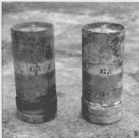
6 lb Ground Bombs :- as recovered Used for small area denial: issued to Home Guard.
