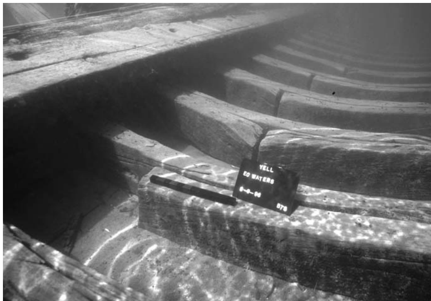
Fig. 2.51 E. C. Waters' frames. View aft of paired frames with butt joints in the wreck's forward port section. The main and sister keelsons overlay the frames in the upper left. Scale = 1 ft. NPS photo by Brett Seymour
