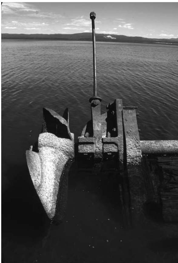
Fig. 2.63 View north, starboard side of adjustable stern bearing assembly ( center ) and propeller ( left ). NPS photo by John Brooks
