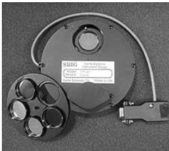
Fig. 13. SBIG STMEI 8 filter wheel and carousel (SBIG, 2003).
