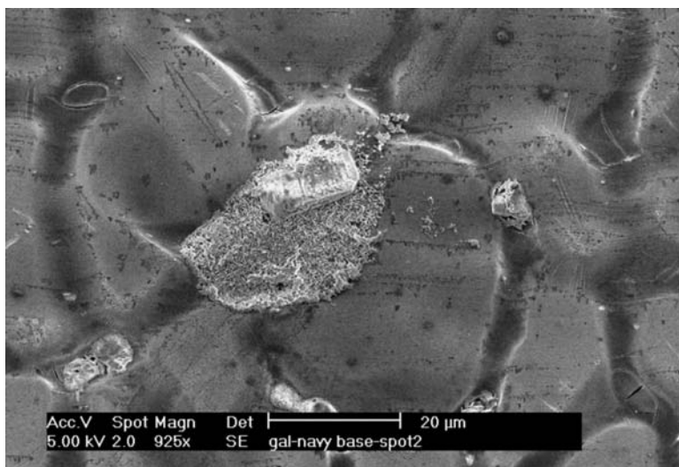
Fig. 14. SEM micrograph showing increased activity between salts and a galvanized steel surface at grain boundaries and triple points.
