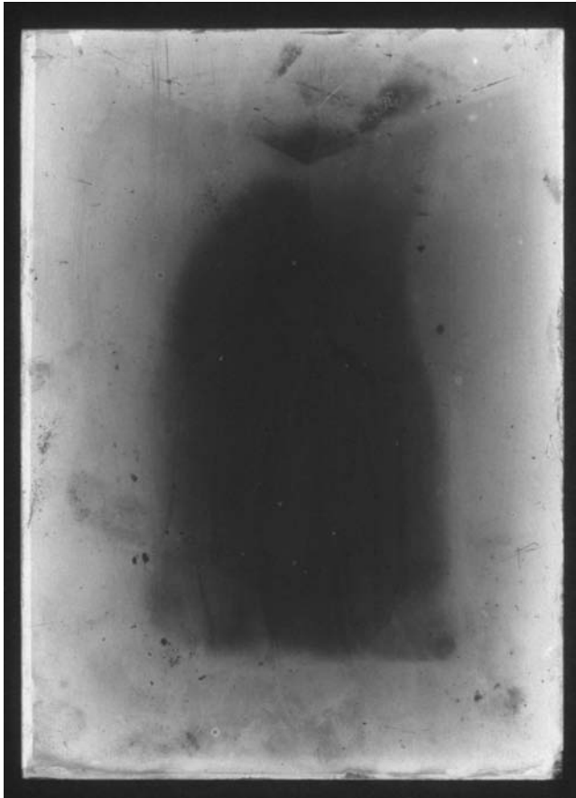
Fig. 4. Silver gelatin glass negative. Cueni study collection (~1910). The mirroring stain is wide, partially obscuring the image.
