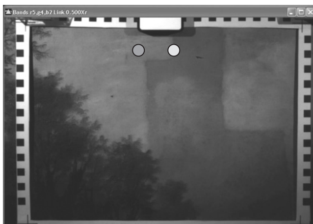
Fig. 53. Partially removed varnish with tested areas (blue dot = cleaned area, yellow dot = aged varnish).
