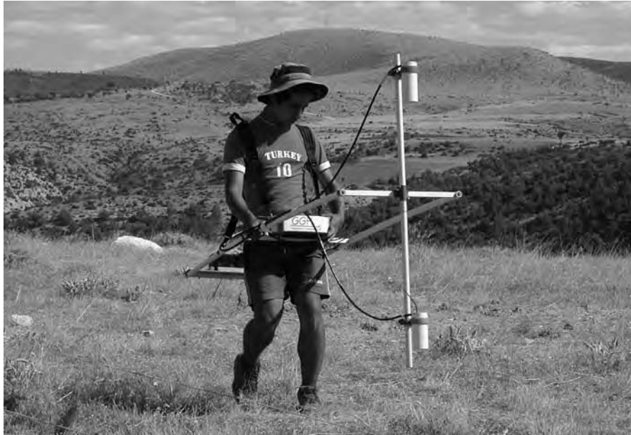
Fig. 8.2 Geomagnetic screening (Ömerçalı in background)
