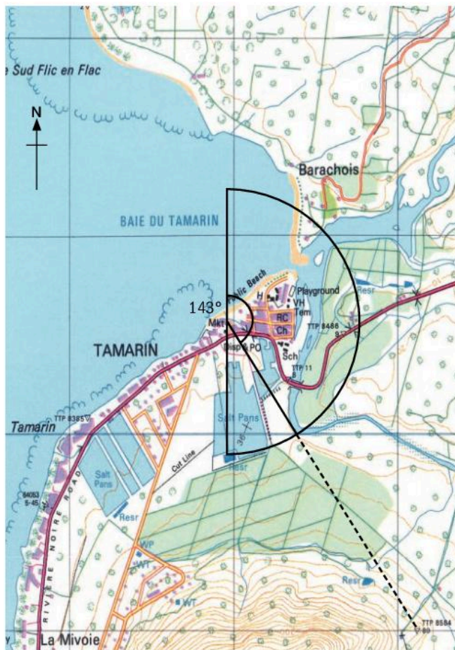
Fig. 12.18 How to use a protractor to measure bearings between 0° and 180°
