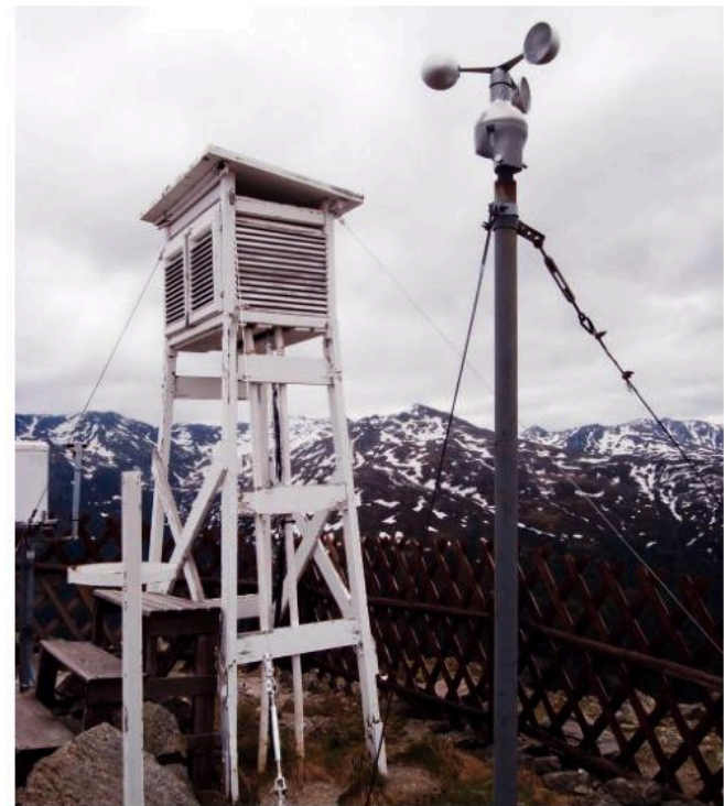
Fig. 6.14 A Stevenson screen located at a weather station in the Austrian mountains
