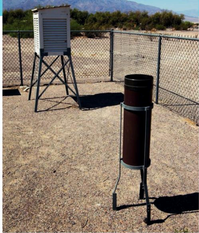
Fig. 6.13 A Stevenson screen located at a weather station in Death Valley, USA (a hot desert area)
