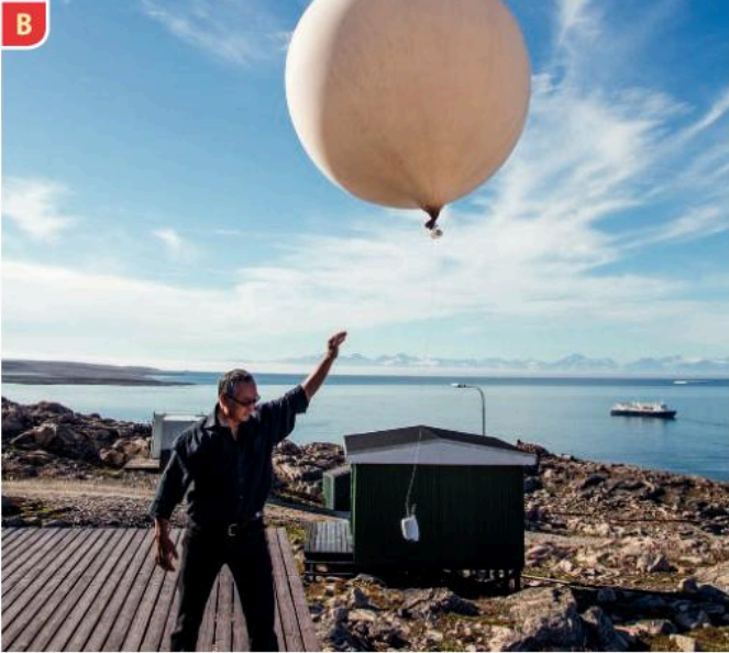
▲ Four times a day, weather balloons are launched from six sites in the UK. The little package collects and transmits data.
