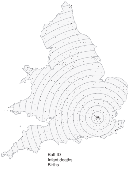
(c) Overlaying (a) and (b) produces a new point layer
