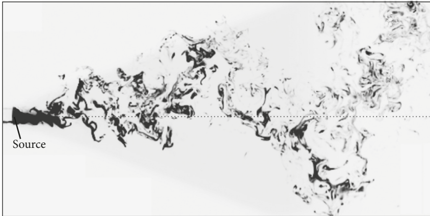
Figure 3.32 Odor plume in a turbulent environment. Shown here is a two-dimensional section through a plume created when a tracer substance is injected into a turbulent stream of water. It mimics the formation of an odor plume in turbulent air. In both cases, the plume doesn't form a continuous concentration gradient but, instead, breaks up into discontinuous packets.
