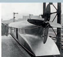
**Rear fairing** The wind-tunnel-designed fairing had a four-bladed propeller made of ash wood.
