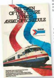
The turbo train Amtrak introduced six 125-mph (201-km/h) Turboliner trains from 1973 on services from Chicago. Powered by Turbomeca gas turbines originally designed for helicopters, the trains never got to exploit their highspeed capability.
