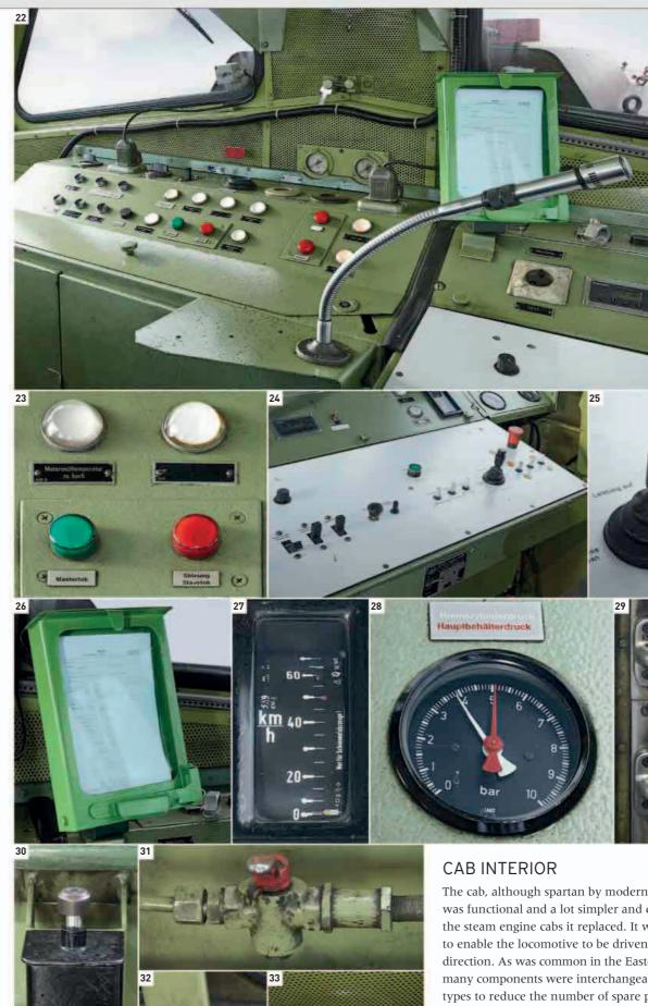
The cab, although spartan by modern standards, was functional and a lot simpler and cleaner than the steam engine cabs it replaced. It was designed to enable the locomotive to be driven in either direction. As was common in the Eastern Bloc, many components were interchangeable with other types to reduce the number of spare parts required.
