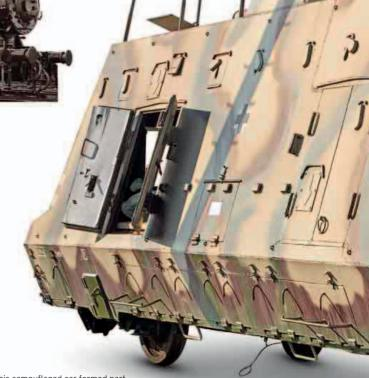
This camouflaged car formed part of a German Wehrmacht BP42 armoured train that protected supply and transport trains in the Balkans and Russia. An armoured Class 57 0-10-0 steam locomotive was positioned in the centre of the train, which consisted of a combination of infantry, navigating, anti-aircraft, and artillery wagons, with converted tank turrets
