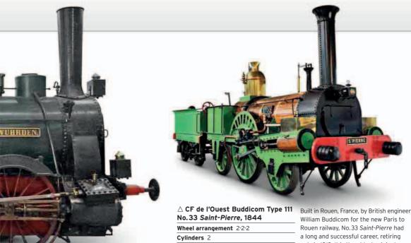
Boiler pressure 80 psi (5.62 kg/sq cm) Driving wheel diameter 75 in (1,905 mm)
