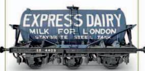
**London's dairy supplier** With a capacity of 3,000 gallons (13,638 litres), the Express Dairy six-wheel milk tank wagon weighed as much as a loaded passenger coach when full. This wagon was built by the Southern Railway in 1931 and rebuilt in 1937.
