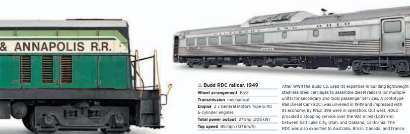
stainless-steel carriages to assemble diesel railcars (or multiple units) for secondary and local passenger services. A prototype Rail Diesel Car (RDC) was unveiled in 1949 and impressed with its economy. By 1962, 398 were in operation. Out west, RDCs provided a stopping service over the 924 miles (1,487 km) between Salt Lake City, Utah, and Oakland, California. The RDC was also exported to Australia, Brazil, Canada, and France.
