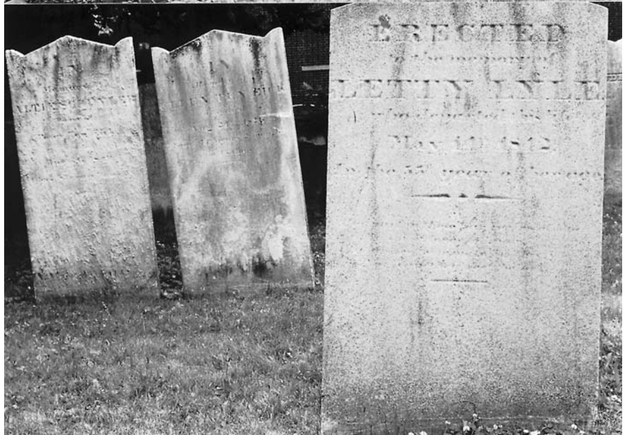
The grave marker at top is dated 1804, and the words are still clearly inscribed in the resistant stone. In contrast, the limestone grave marker from 1812 ( bottom ) is difficult to read because acid weathering has blurred the lettering. (Photographs courtesy of MACGES.)
