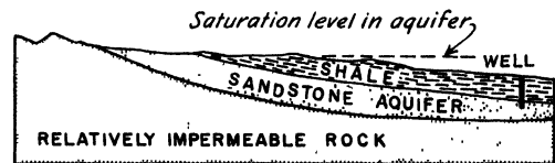
FIG. 16.19 (Above) A structural artesian condition such as that described in the northern Great Plains of the United States. (Below) A local artesian condition that might occur in an area of glacial deposition.
