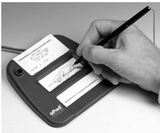
Figure 6. Example of electronic pad system accepting written signature for digitalization process in electronic signature-based applications
