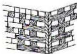
Fig. 62 Corner Timbering at Karanis.
