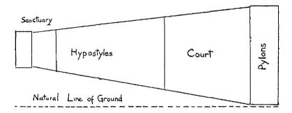
Fig. 74.—Ground and Roof-lines of the Temple.
