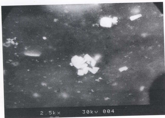
Figure 8.6 Photomicrograph of calcium antimonate crystals in opaque white fourteenth-century BC Egyptian glass (magnification \times 2,500 ).
