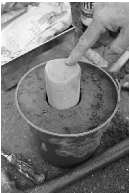
Figure 4.4 A tubular-shaped mould in sand, ready for filling with molten copper
