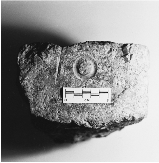
Figure 3.18 An experimental groove in rose granite, cut with a pointed, 'trifacial' flint tool
