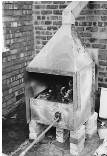
Figure 2.48 The author's furnace for melting copper and bronze
