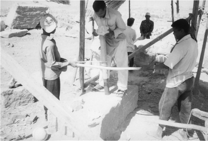
Figure 4.21 In the foreground, the team of three workers is drilling a block of rose granite with an 8 cm-diameter copper tube. In the background, two sawyers operate the flat-edged copper saw
