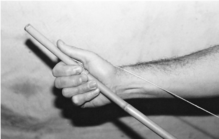
Figure 8.22 The thumb placed between the bow-string and the bow-shaft, which automatically adjusts the string's tension during drilling
