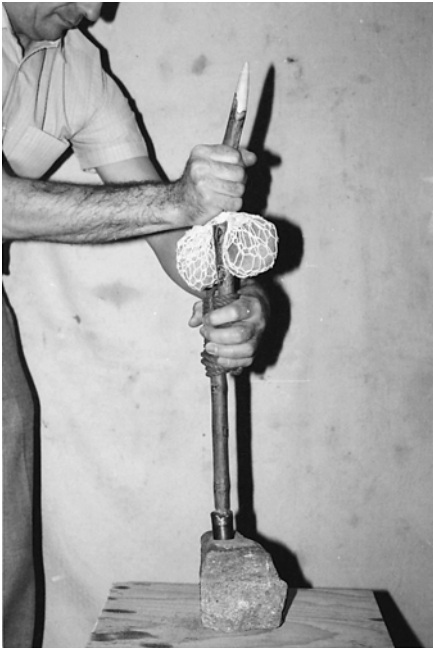
Figure 5.16 A reconstructed TRTD, weighted with two stones, driving a copper tubular drill
