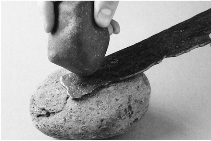
Figure 2.28 Beating a reconstructed copper saw casting to shape on a stone anvil with a stone hammer
