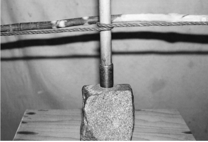
Figure 4.8 Drilling diorite with a bow-driven bronze tube and sand abrasive
