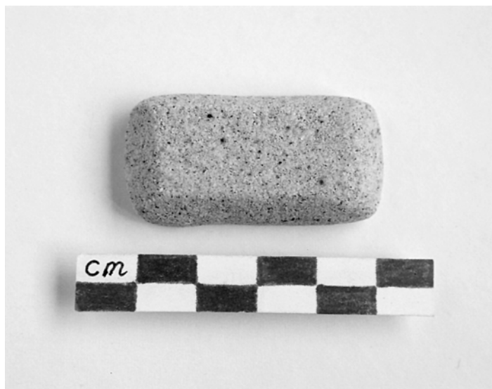
Figure 9.2 A test core, made from hard limestone-derived powder
