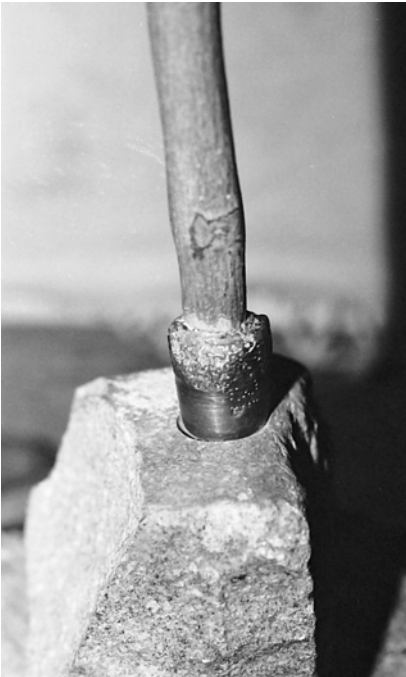
Figure 4.9 Close-up of a copper tubular drill, engaged in the drill-hole. Notice that the hole is slightly overcut due to the lateral forces imposed during the drilling action
