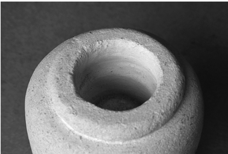
Figure 5.34 The groove ready for admitting a borer
