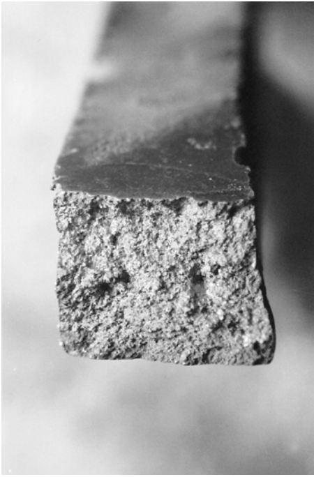
Figure 2.51 A fractured bronze casting caused by extreme hammering
