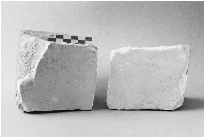
Figure 7.17 Two small limestone blocks, each with a surface flattened to a tolerance of 0.25 mm
