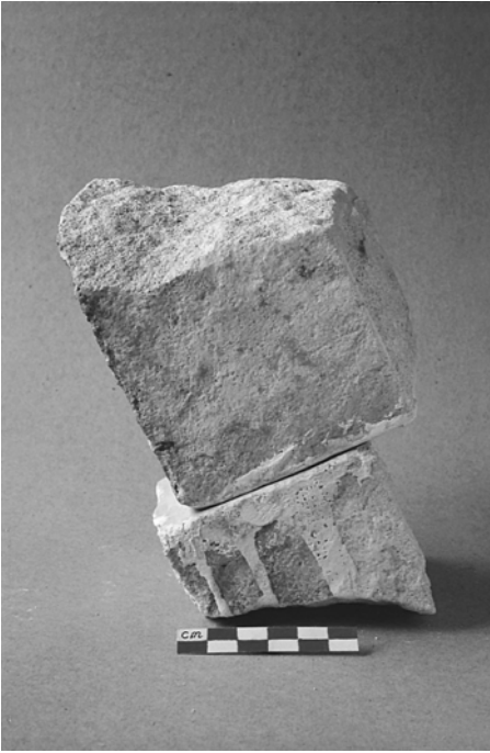
Figure 7.18 The lubricated sliding test using the prepared limestone blocks
