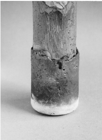
Figure 5.18 A 7 cm-diameter cast copper drill-tube, fitted to the lower end of a TRTD central shaft
