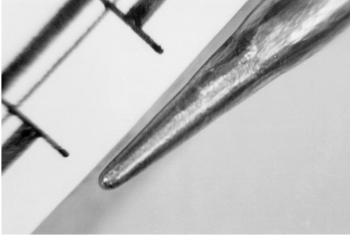
Figure 8.23 A close-up view of a bronze rod's drilling point
