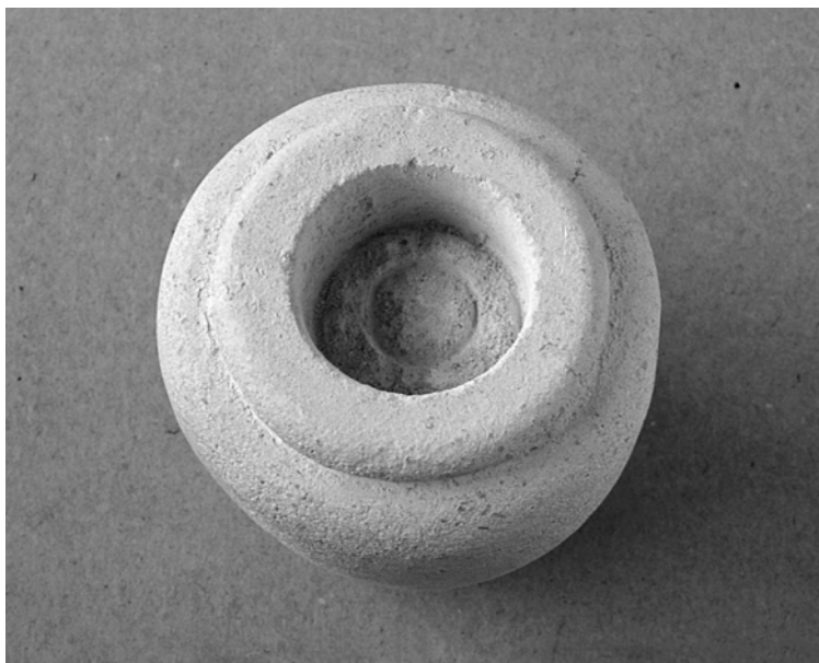
Figure 5.32 The tubular core is now removed
