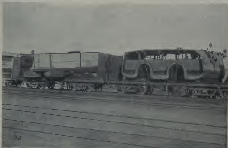
TRANSPORT OF SECTIONS OF LORD KITCHENER'S GUNBOATS BY RAILWAY.
