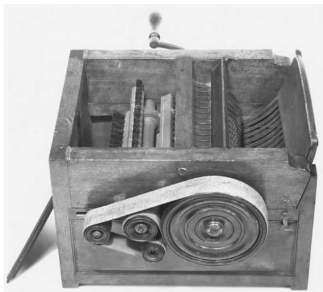
Replica of Eli Whitney's cotton gin, invented in 1793. This machine for cleaning the seeds out of cotton helped make cotton the main crop of the American South and kept slavery as its dominant economic institution. © Bettmann/Corbis
