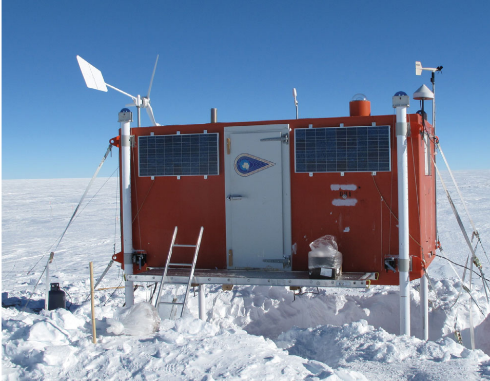
Figure 7.7 The wind and solar powered US Automatic Geophysical Observatory (AGO). These remote platforms on the Antarctic plateau consist of a suite of instruments used to monitor the space environment of Earth over a range of radio and optical wavelengths. Real-time data acquisition via satellites enables forecasting and now-casting capabilities for space weather applications. Although the AGOs were originally intended as space physics platforms (optical and radio wave auroral imagers, magnetometers and narrow- and wide-band radio receivers), the reliability and flexibility of the design has enabled other disciplines to leverage the location and infrastructure for new scientific instruments including seismometers, comprehensive weather stations and astrophysical sensors.
