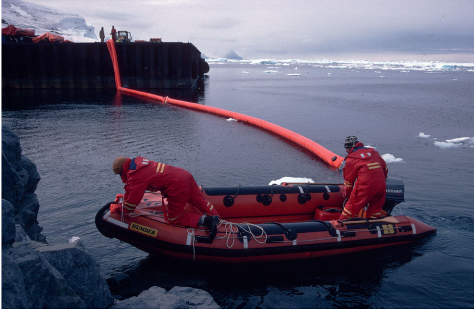
Figure 10.11 Marine pollution exercise, deploying an oil boom at Rothera Research Station. (Credit: Peter Bucktrout , BAS)
