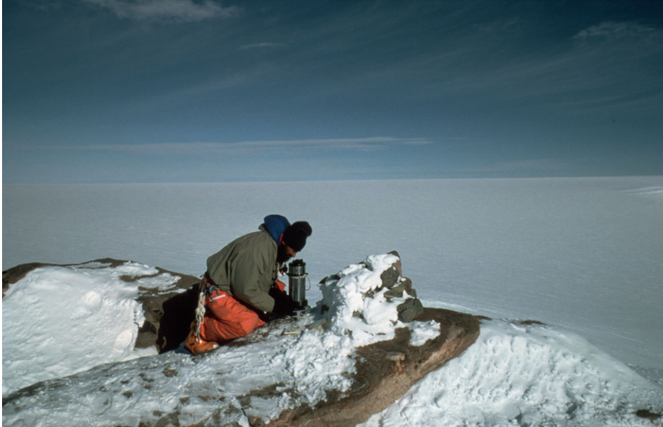
Figure 2.23 Geophysicist reading a gravimeter at Haag Nunataks, an isolated exposure of Precambrian rock. (Credit: BAS)
