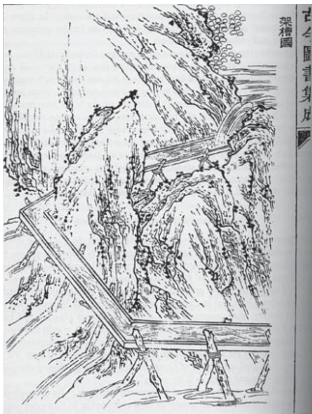
Illustration of an irrigation flume constructed in wood. Such flumes, along with dikes and irrigation canals, would be used for agriculture, particularly for the cultivation of rice. From the Tu Shu Ce Zheng .
