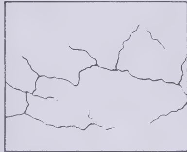
4. EARTH CRACKS 10 Feet
