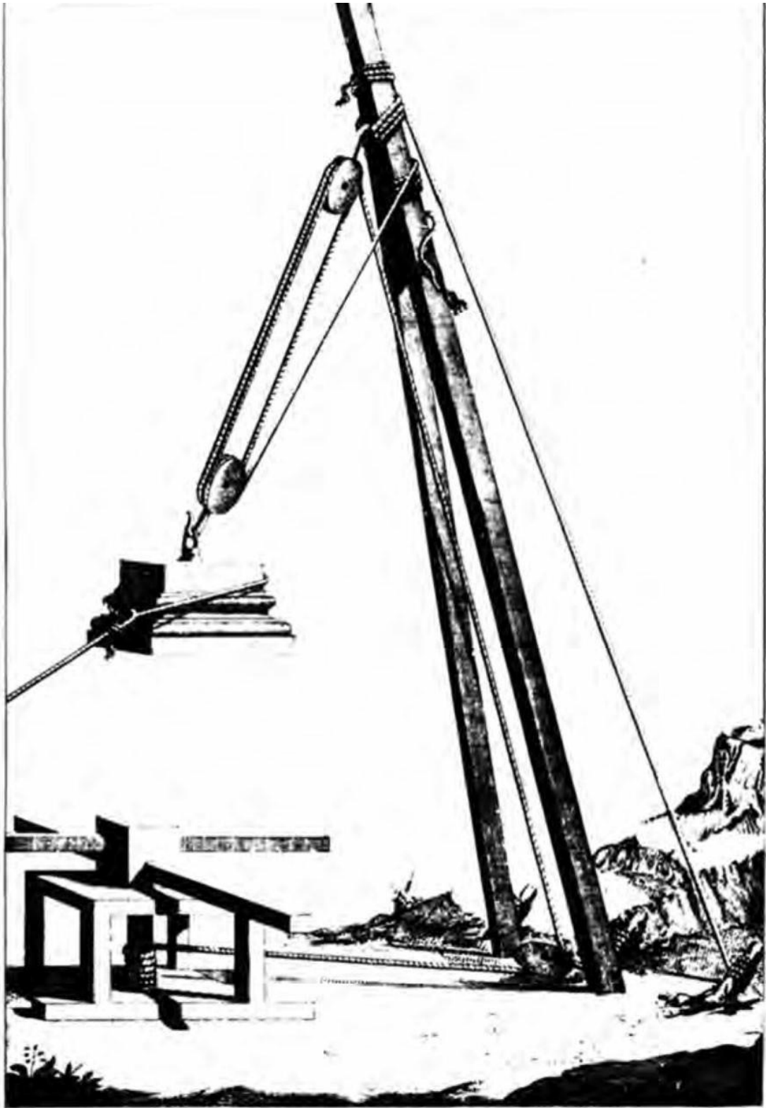
A drawing of the theoretical use of pulleys by the Romans to build Baalbek.
