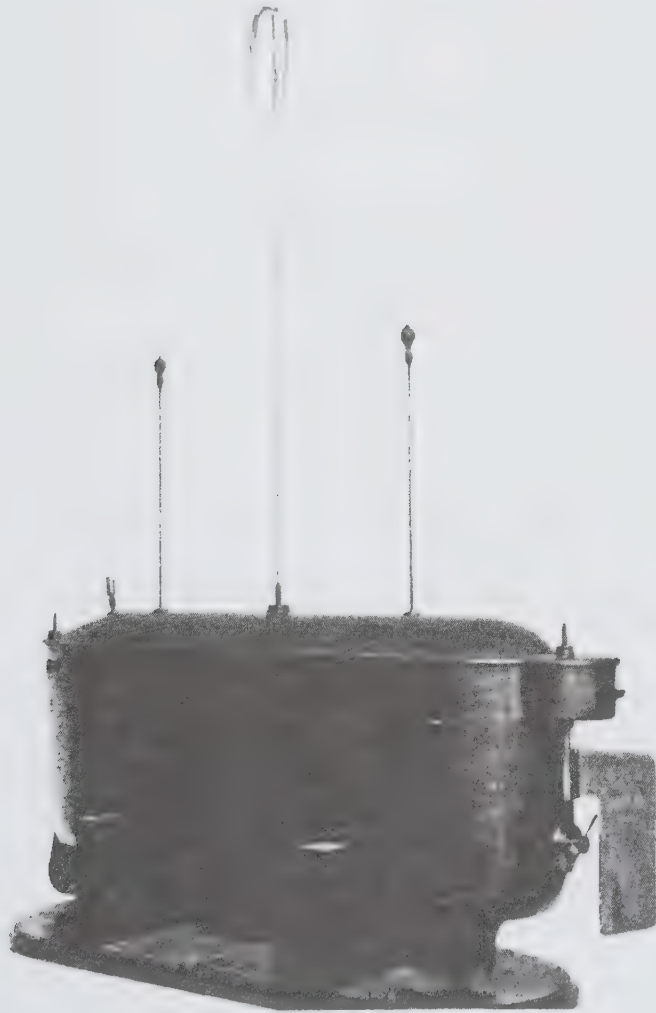
Figure 2. The first practical Telautomaton. A machine having all its bodily or translatory movements and the operation of the interior mechanism controlled from a distance without wires. The crewless boat shown in the photograph contains its own motive power, propelling and steering machinery, and numerous other accessories, all of which are controlled by transmitting from a distance, without wires, electrical oscillations to a circuit carried by the boat and adjusted to respond only to these oscillations.
