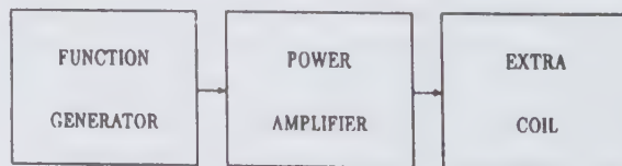
Figure 2. Extra Coil Driven by Power Amplifier
