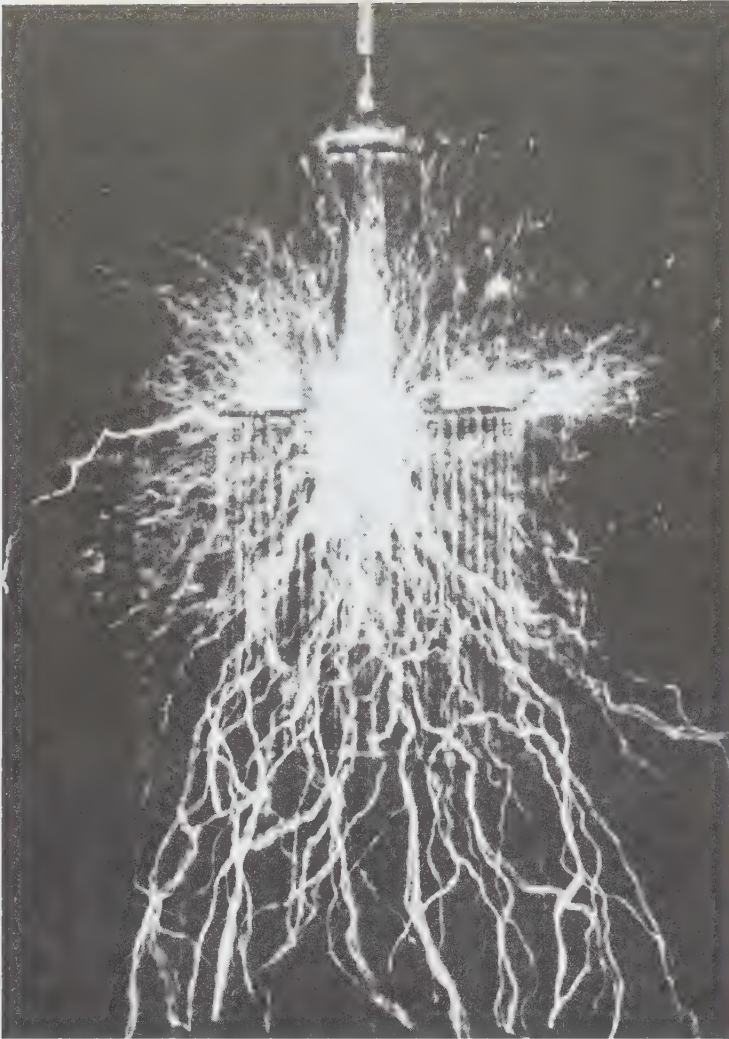
Figure 10. Photographic view of an experiment to illustrate an effect of an electrical oscillator delivering energy at a rate of 75,000 horse-power. The discharge, creating a strong draft owing to the heating of the air, is carried upward through the open roof of the building. The greatest width across is nearly seventy feet. The pressure is over twelve million volts, and the current alternates one hundred and thirty thousand times per second.
