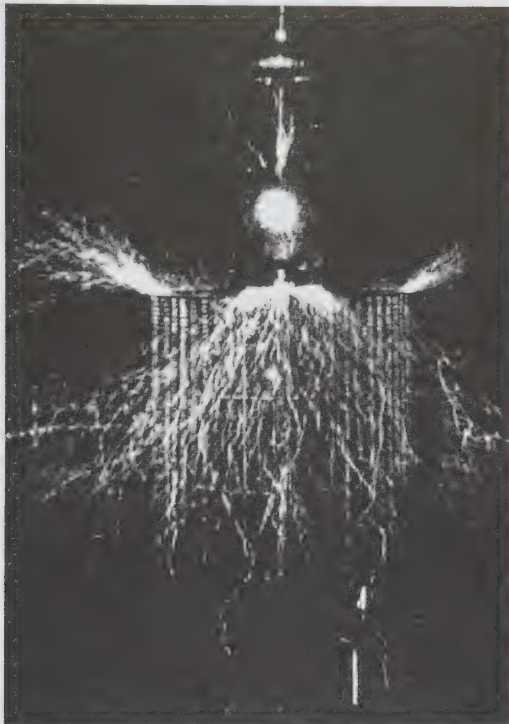
Figure 9. Experiment to illustrate the capacity of the oscillator for creating great electrical movement. The ball shown in the photograph, covered with a polished metallic coating of twenty square feet of surface, represents a large reservoir of electricity, and the inverted tin pan underneath, with a sharp rim, a big opening through which the electricity can escape before filling the reservoir. The quantity of electricity set in movement is so great that, although most of it escapes through the rim of the pan or opening provided, the ball or reservoir is nevertheless alternately emptied and filled to overflowing (as is evident from the discharge escaping on the top of the ball) one hundred and fifty thousand times per second.
