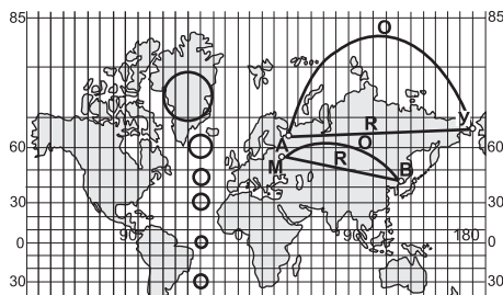
Fig. 205. Mercator map projection: O – orthodromic line, R – rhumb line
