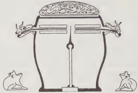
Sketch of Heng's Second Century A.D. seismograph. An earthquake would dislodge one of the balls, which would then fall into the mouth of one of a circle of waiting frogs, thereby providing the direction of the epicenter. (X8)
