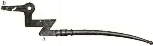
FIG. 54.—SIDE VIEW OF THE TRIGGER OF THE CROSSBOW.
