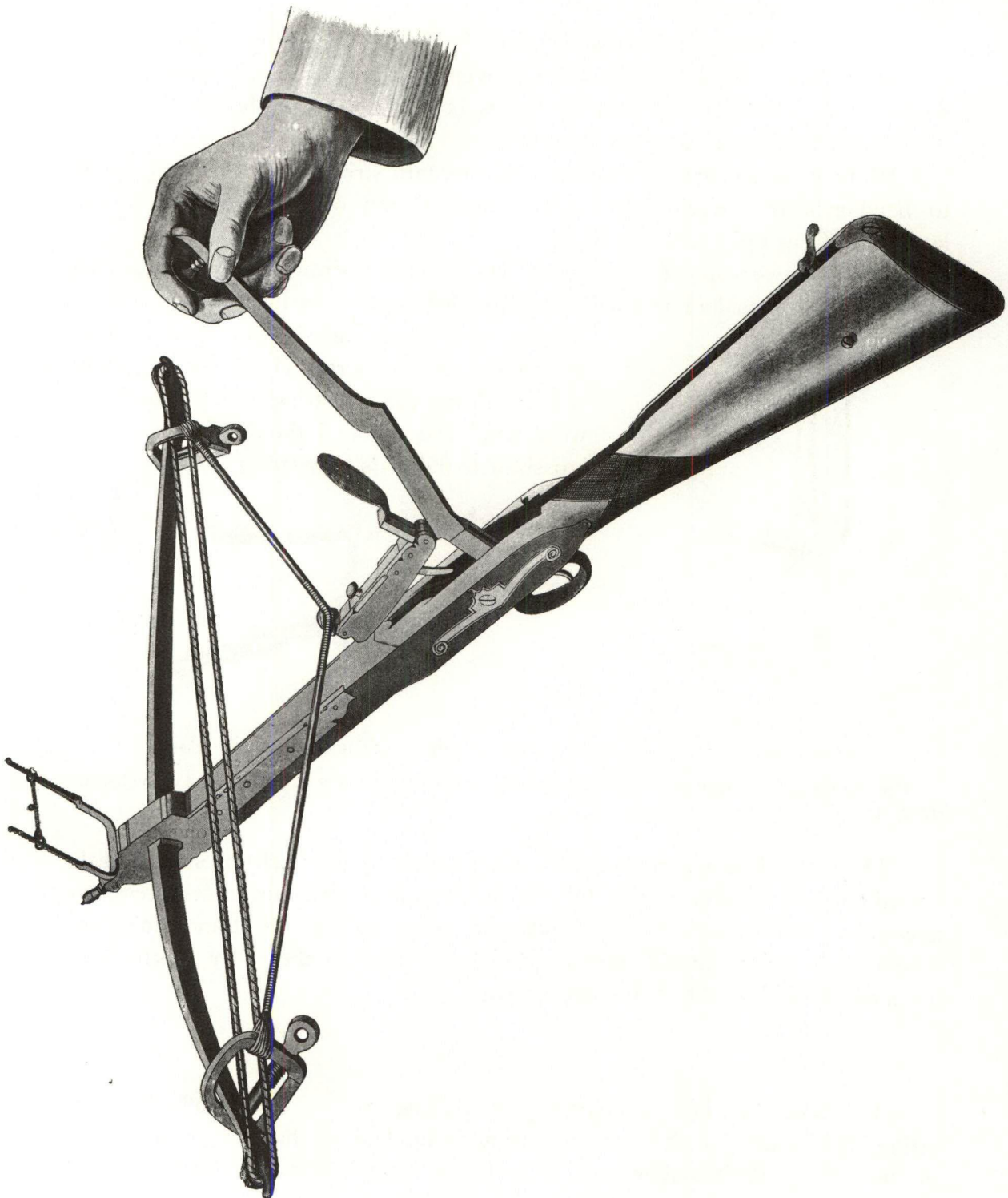
FIG. 122.—THE CROSSBOW BENT SUFFICIENTLY BY THE RASTAD SPRING FOR THE CROSSBOW.
