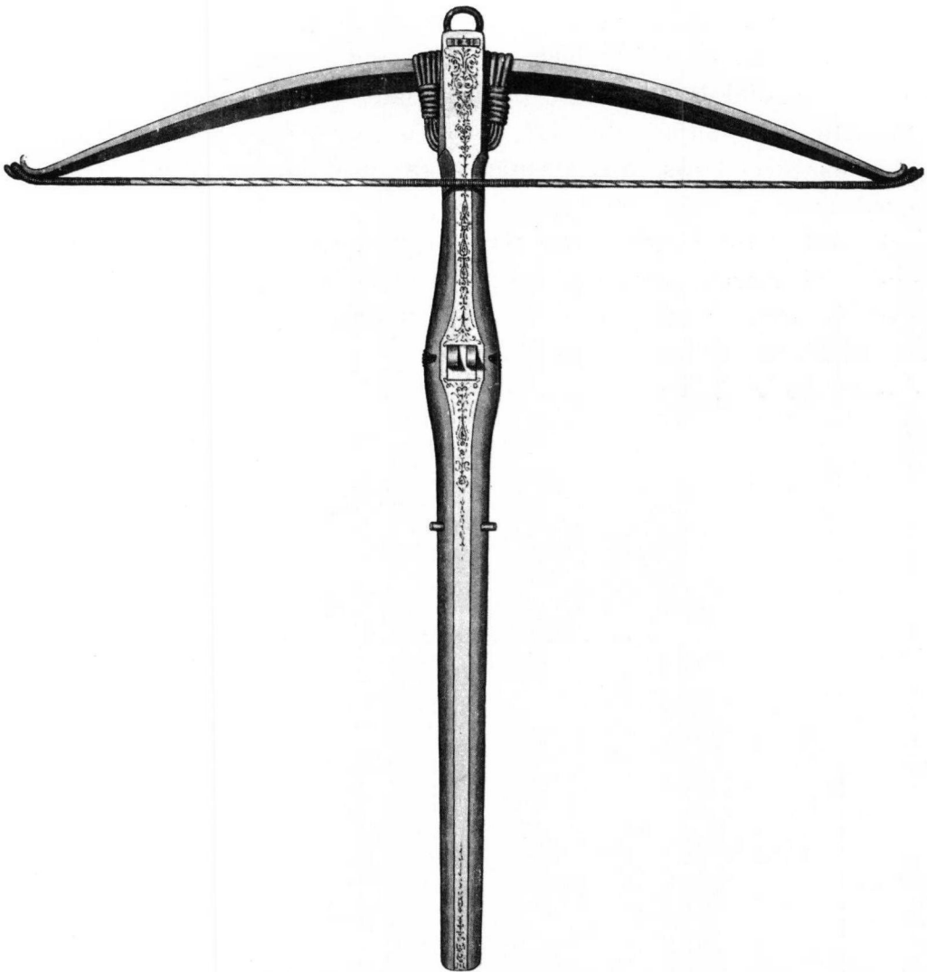
FIG. 27.—A SIXTEENTH CENTURY SPORTING CROSSBOW THAT WAS BENT WITH A CRANEQUIN, AND WHICH HAD A STEEL BOW ATTACHED TO THE STOCK BY A BRIDLE OF SINEW. (Spanish.)
