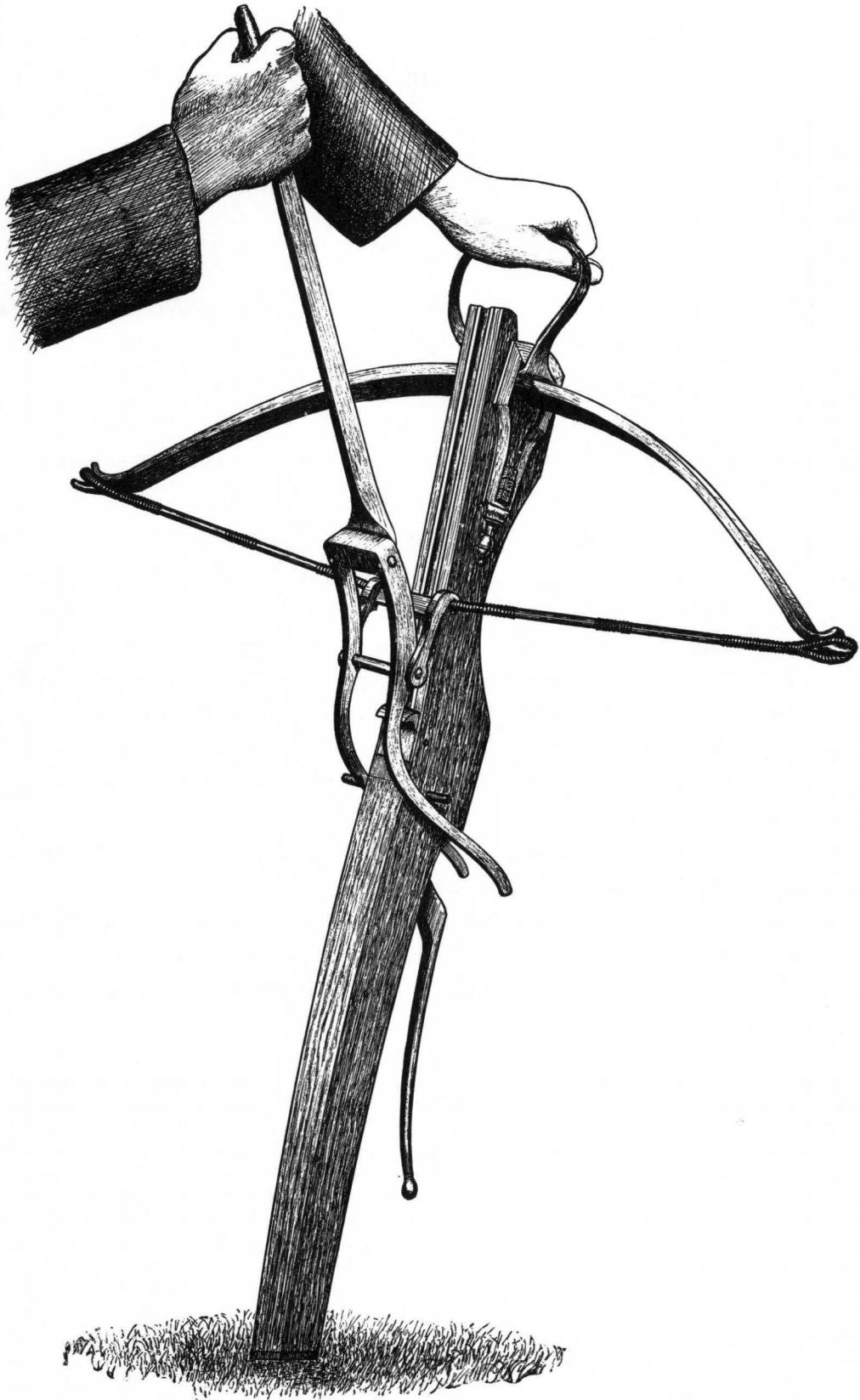
FIG. 45.—A MILITARY CROSSBOW BEING BENT BY A GOAT'S-FOOT LEVER.
