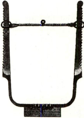
FIG. 141.—THE FORE-SIGHT, WITH THE SIGHTING BEAD ON ITS SKEIN.
