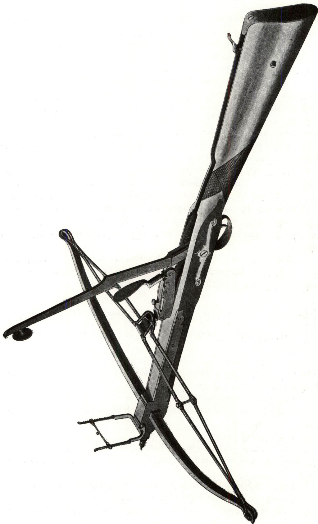
FIG. 116. -THE STRING ON THE CATCH OF THE LOCK AND THE LEVER HINGED FORWARD READY TO BEND THE BOW.
