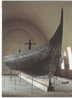
The Gokstad ship, a 76ft (23m) Norwegian oak vessel, carried sixty-four warriors. Although its shallow draught made it suitable for rivers, a replica was sailed across the Atlantic in 1893.
