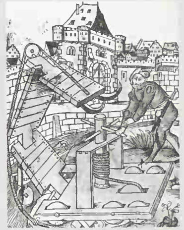
Above. Collapsible drawbridge used for defense (Bellifortis, Conrad Kyser's treatise on warfare, 1405).
