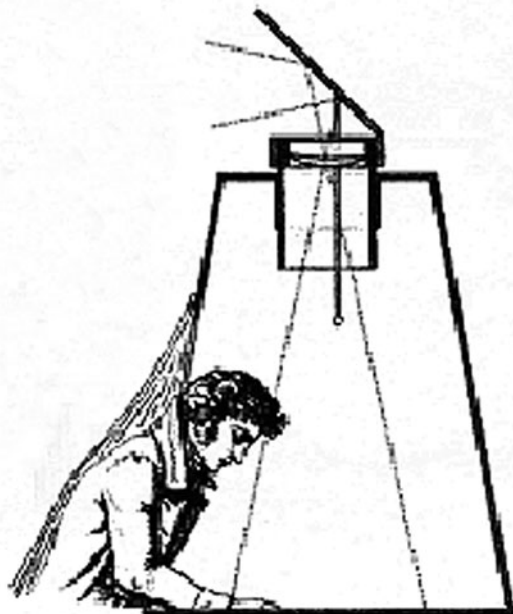
Fig. 5.1 The device Biot referred to as a “ chambre noire .” (From Biot, Traité .)
