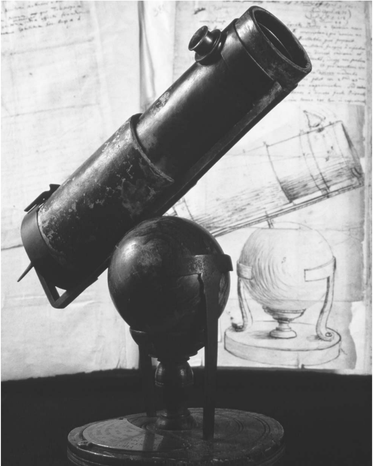
Scientific Instruments. Isaac Newton's telescope, the first reflecting telescope, made in 1668, in front of a corresponding drawing from the Principia Mathematica . ©JAMES A. SUGAR/CORBIS
