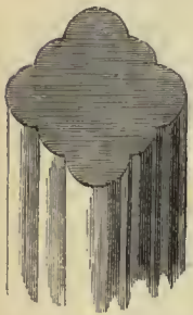
643.—Section of Shaft, Exeter.
