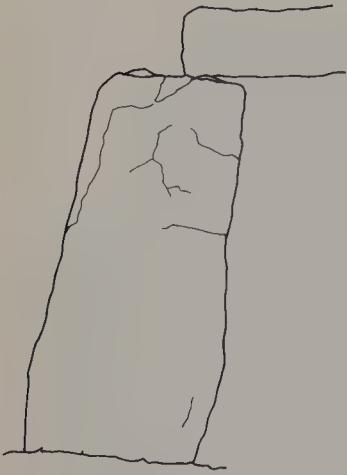
267 The archive records changes in modern as well as ancient Stonehenge. In this 1919 Ministry of Works drawing, stone 4 is leaning and putting both itself and the lintel it supports at risk.
