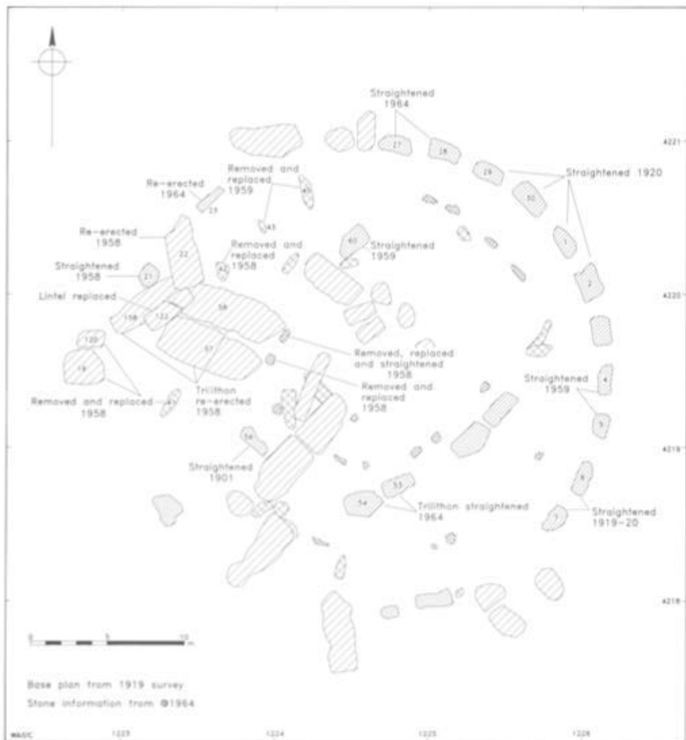
Fig 188 Plan of the stones showing those fallen in 1919 with information on restoration
