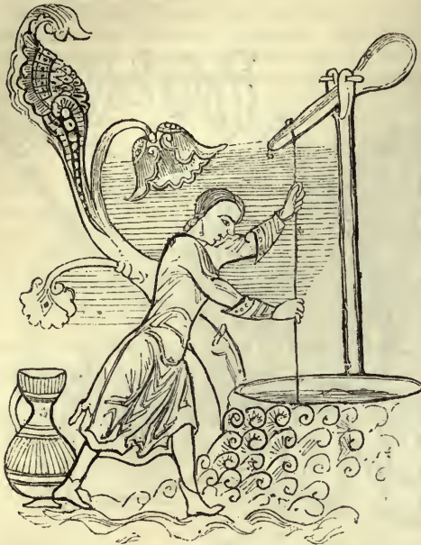
RAISING WATER FROM A WELL WITH A LOADED LEVER. Cotton MS. Nero, C 4.
