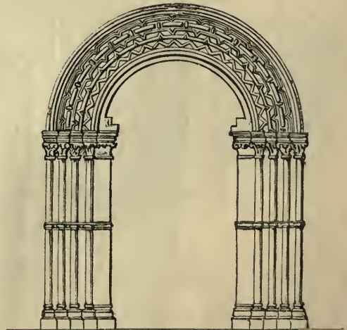
DOOR-WAY OF ST. LEONARD'S CHAPEL, STAMFORD. This door was originally square, as may be seen by the abutments of the flat arch.
