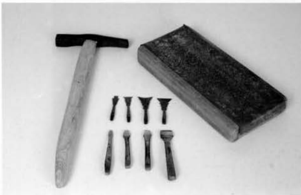
Reproduction pinking tools by Dan Brown ( www.greenmanforge.com ) and Dave Hodgson ( www.bodgeramour.co.uk ). A lead-covered block is placed under the fabric to preserve the blade's edge.
