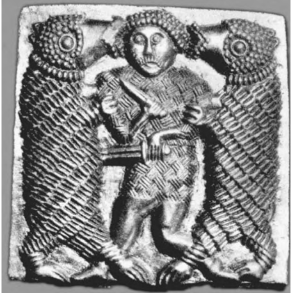
Die for stamping the decorative plaques on seventh-century Swedish helmets. (Statens Historiska Museum, Stockholm)
