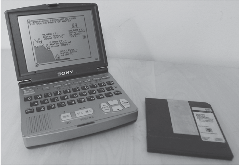
Figure 10.1 Sony's Data Discman displaying material from Compton's Concise Encyclopedia . When folded, the Discman measured around thirteen by ten by three centimeters. The disc on the right is for the New Grolier Electronic Encyclopedia . Photograph courtesy of Nate Hoffelder, The Digital Reader ( www.the-digital-reader.com ).
