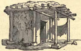
FIG. 19.—Primitive hut of mud and timber framing.
