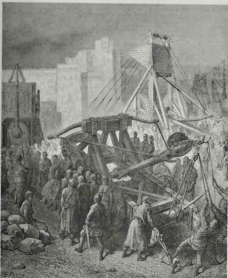
Large catapults are here shown in use during the storming of a crusader fortress. Note the men in the foreground turning a winch to increase the tension on the device's throwing arm.
