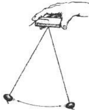
Figure 8.1. A basic pendulum is a very accurate tool to measure time.
