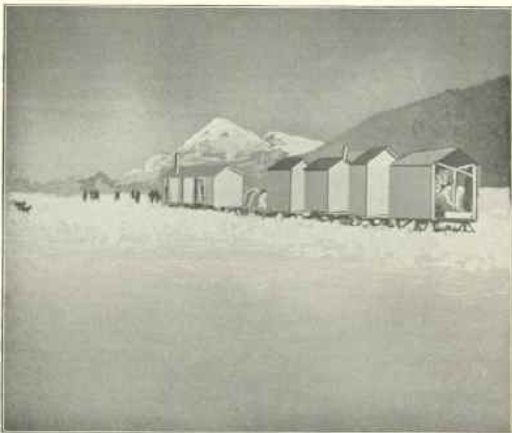
STEAM LOCOMOTIVE ON RUNNERS—DESIGNED TO DRAW HEAVILY LOADED VANS OVER THE SNOW.
