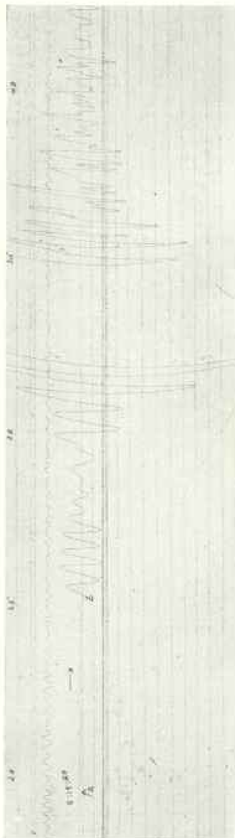
Record of San Francisco Earthquake as made by the Seismograph at the U. S. Weather Bureau, Washington, D. C. East and west component. Numbers at top are minutes of time corresponding to the dots on the record. (See page 296)
