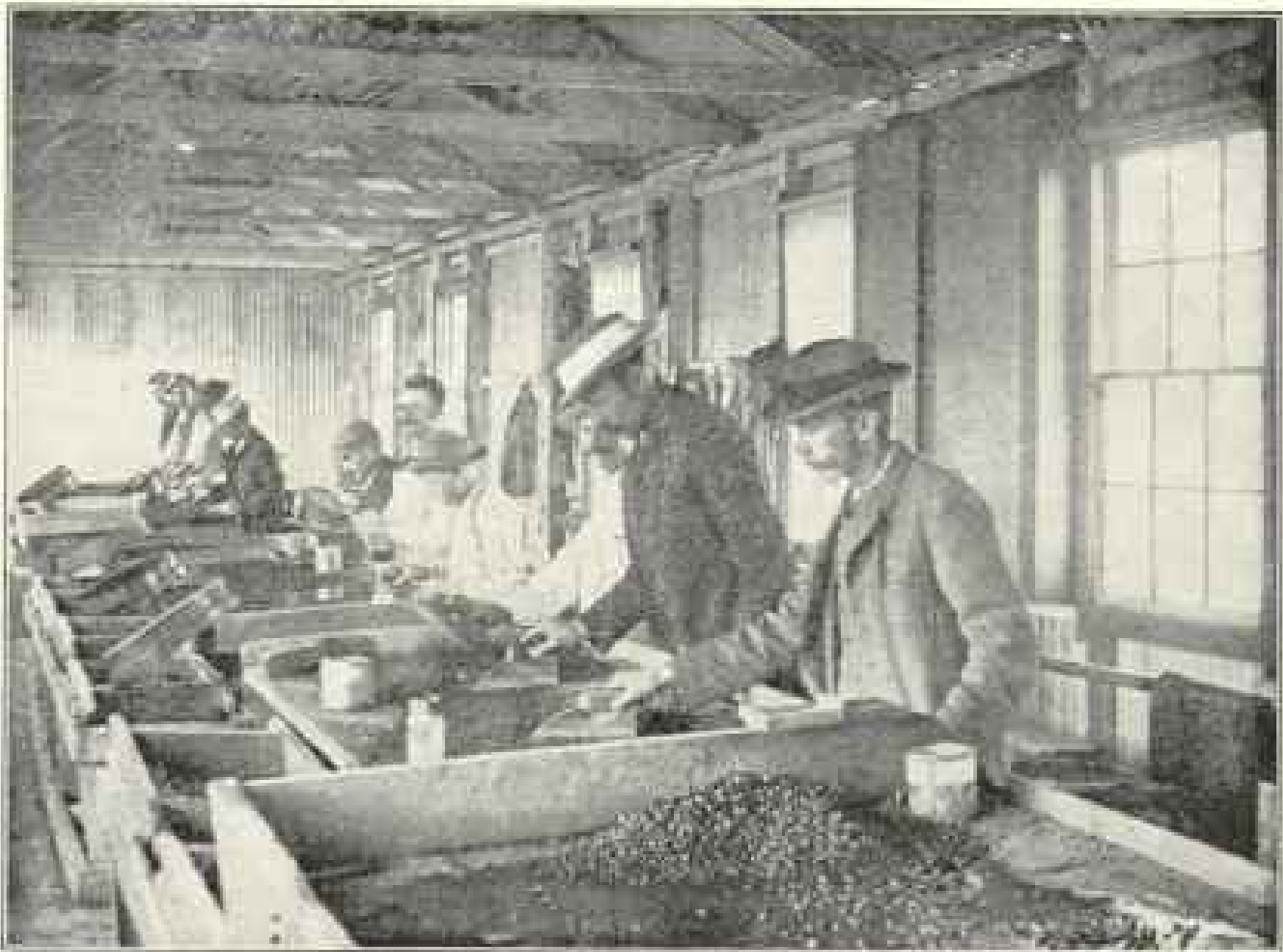
The Old Method of Separating the Diamonds—Picking them out of the gravel by hand.
