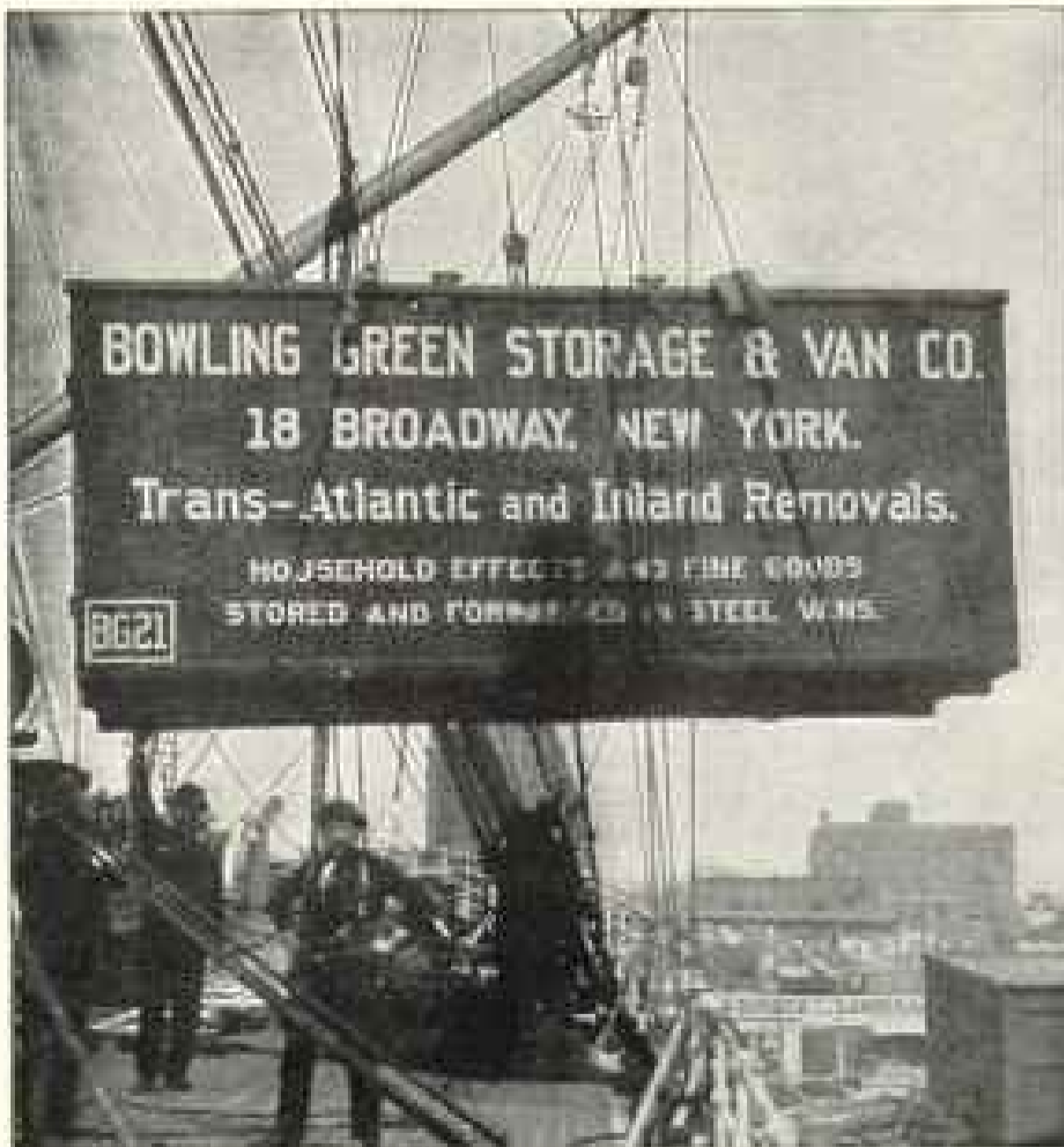
Hoisting Lift-van on Board Steamship
